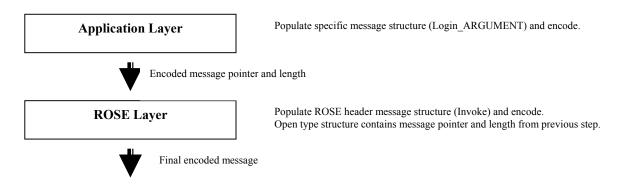
On the decode side, the process would be reversed with the message flowing up the stack:
